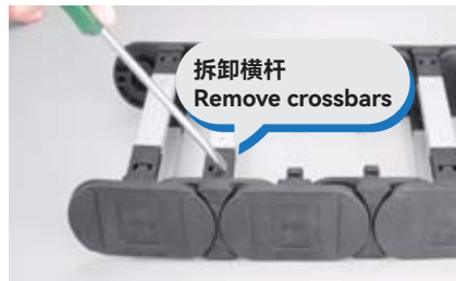
拆卸横杆 Remove crossbars 螺丝刀插入槽中利用杠杆运动撬开横杆 Insert screwdriver into the slot. Using a lever action, release the crossbars
